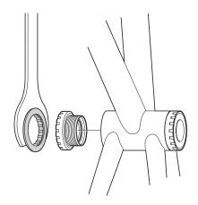
Tightening torque: 35.0 - 50.0 N⋅m {306 - 437 in. lbs.}
