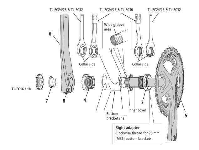
**3.** Check that the inner cover is installed to the right adapter unit, insert the right adapter from the right side of the hanger, and tighten 2 to 3 turns with your hand.
