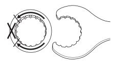
When setting TL-FC24/25 to TL-FC32, check the installable position.
