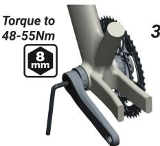
Now, use an **8mm hex torque** wrench and tighten the Non-Drive crankarm bolt to **48-55Nm**.
