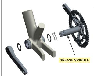
**2** Carefully align the left crankarm so that its internal spline mates with the spindle spline.
