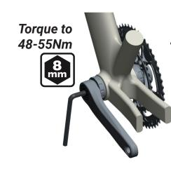
3 Now, use an 8mm hex torque wrench and tighten the Non-Drive crankarm bolt to 48-55Nm.
