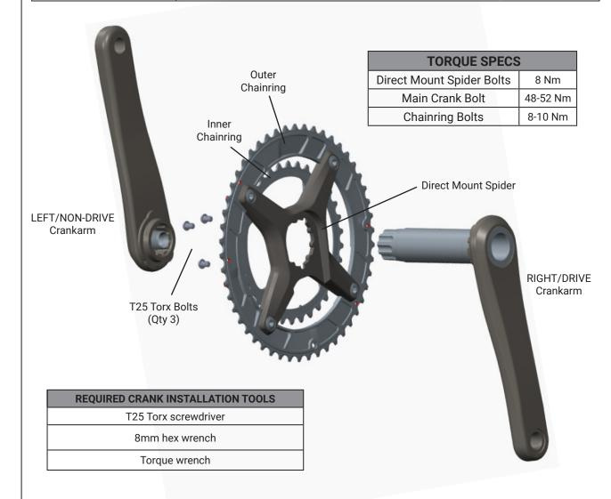
READ THIS FIRST: These are crank installation instructions only. The bottom bracket (sold separately) must already be installed in the frame. Be sure to use only 1 (one) BB Dust Cover (DC) per side during crank installation.
