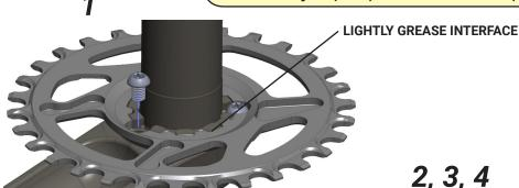
Install Praxis Wave chainring. Lightly grease the ring interface prior to installation to prevent noise. Using the 3 T25 Torx bolts that are in the Right/Drive crankarm install the ring. Bolts must be
