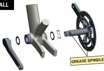
1. Slide the Drive Side Wave Washer onto the spindle.
