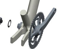
**3.** Use an **8mm hex** torque wrench and tighten the Non-Drive crankarm bolt to **48-55Nm**.
