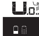
If an eBike has two batteries inserted into it and both batteries are charged on the bike, the charging progress of both batteries will be indicated on the display (the left-hand battery pack is being charged in the illustration). You can also tell by the flashing indicator on the battery which of the two batteries is being charged.
