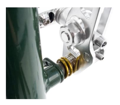
Use a light coat of grease on the cantilever posts and the posts' threads.
