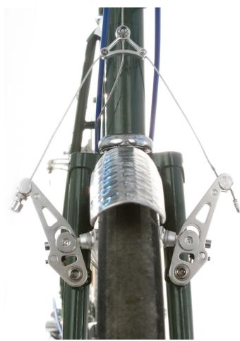
The 13mm nut is for adjusting the pads' height and pitch.
