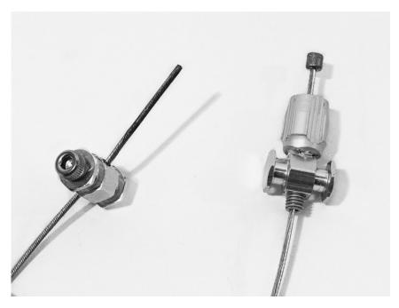
Slip the adjuster over the cable and tighten the anchor.
