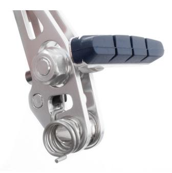
You'll need to install the springs on the brake arms before putting them on the posts. Hook the long end on the adjuster through the cutout in the brake.
