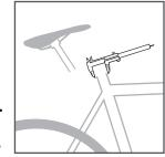
NOTE: The lip of your clamp should be on top so you are comparing the largest diameter of the clamp with the circles below. Make sure there is no tension on the clamp bolt.
