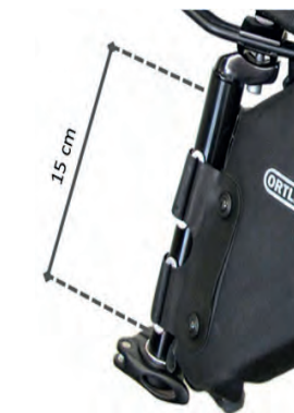
Space required for mounting Seat-Pack 16,5 L to the seat post
