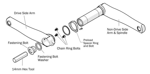
Tools Required: 14mm Socket Wrench (Or Allen Wrench), T25 Torx Wrench, 2.5mm Allen Wrench, Torque Wrench
