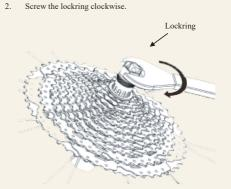
Tighten the lockring with the lockring tool and torque wrench. The tightening torque is 40 N-m.
