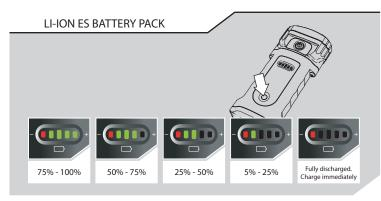
The integrated ES (Energy Status) battery features a 5 stage fuel gauge. Press and hold the 'TEST' button to activate the LED display. This gives a visual indication of the remaining capacity within the battery cells.
