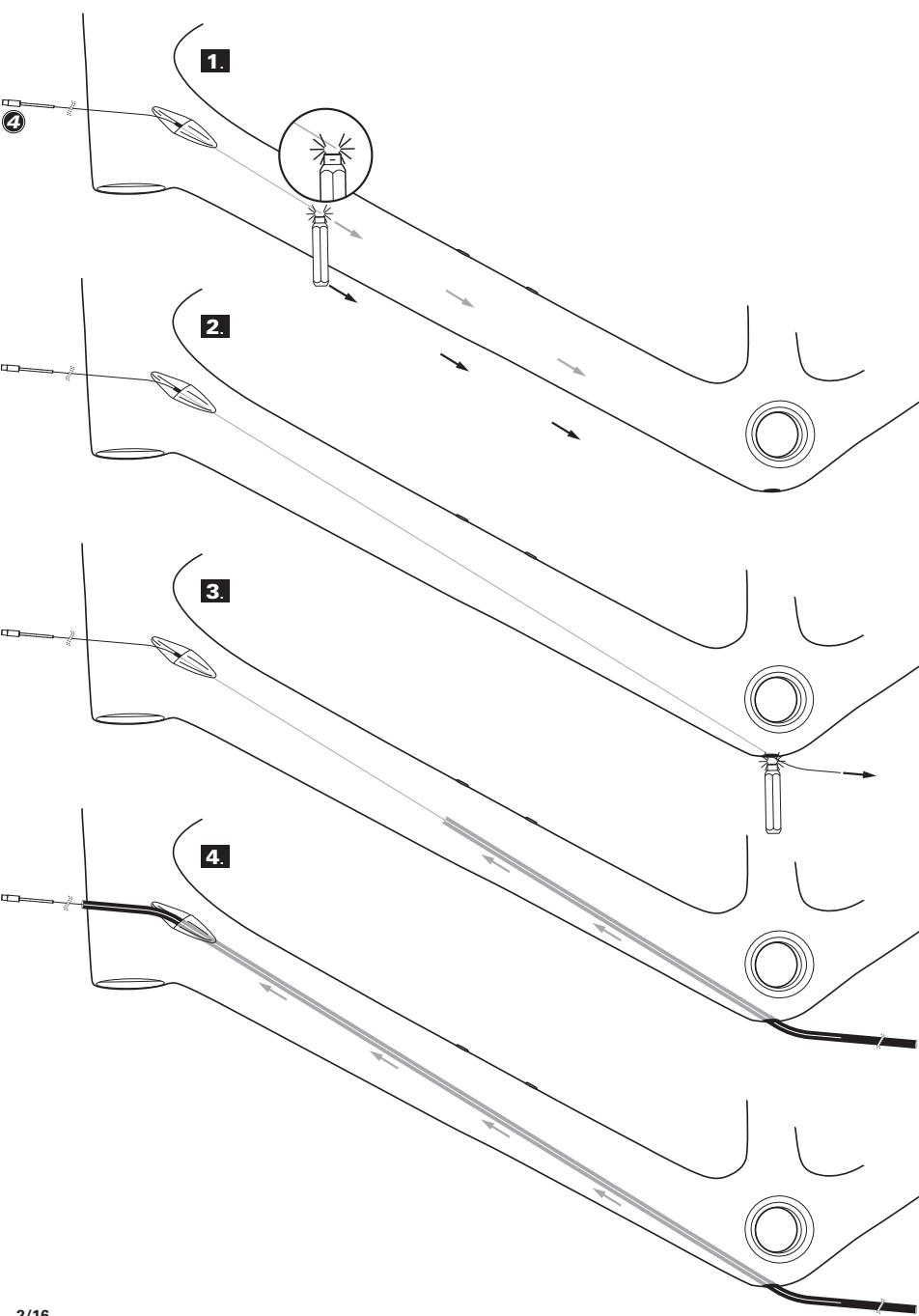
**Method D:** Installing cables with no housing.
