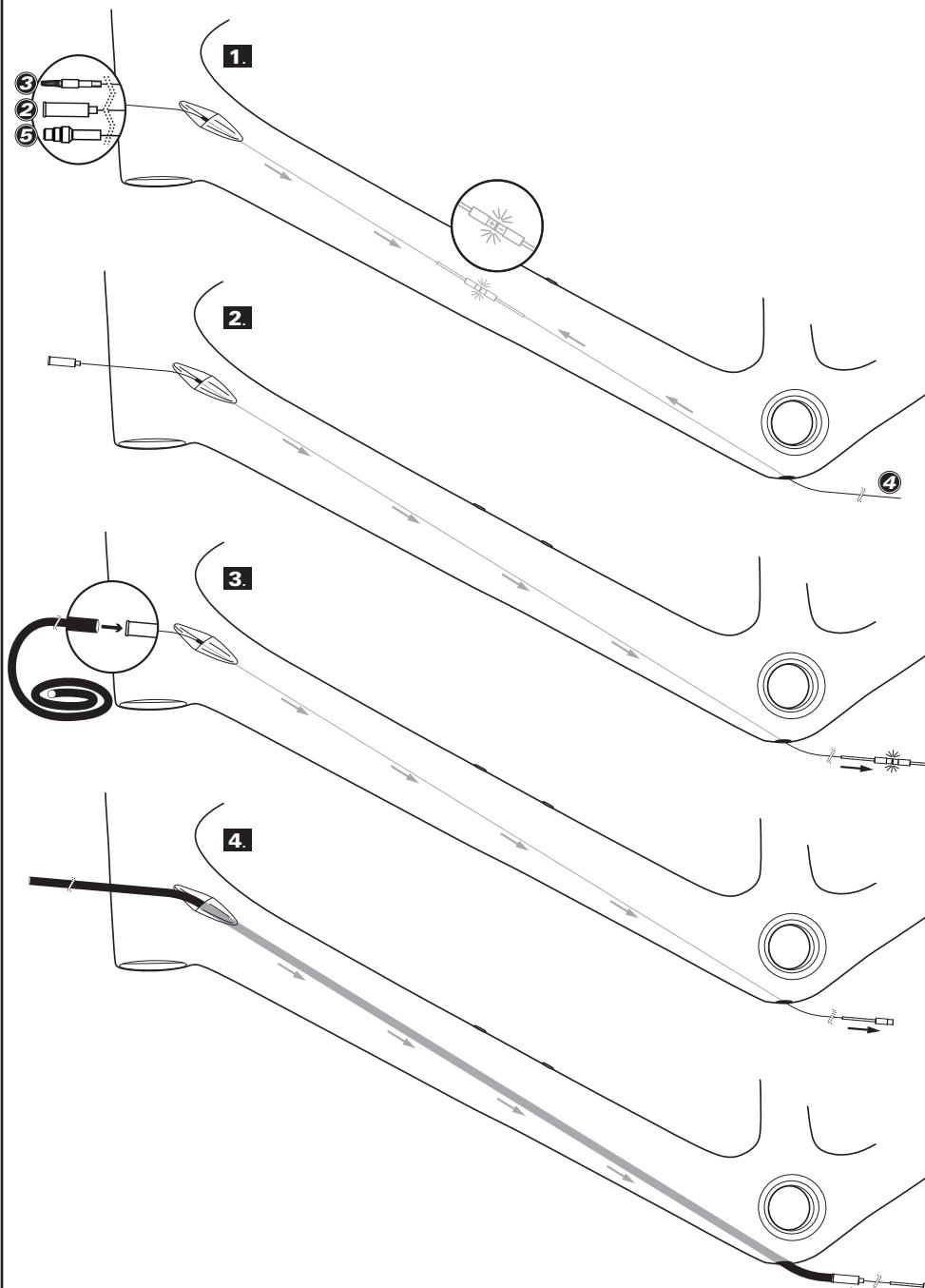
**Method B:** Installing housing, electronic wire and brake line.
