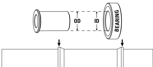
**EN 1. Select Pilot** The pilot helps maintain alignment of the bearing and bushing as the bearing is pressed into the hub shell. 14 pilots (in 7 sizes) are included, each engraved with its outside diameter (OD) and part number.
