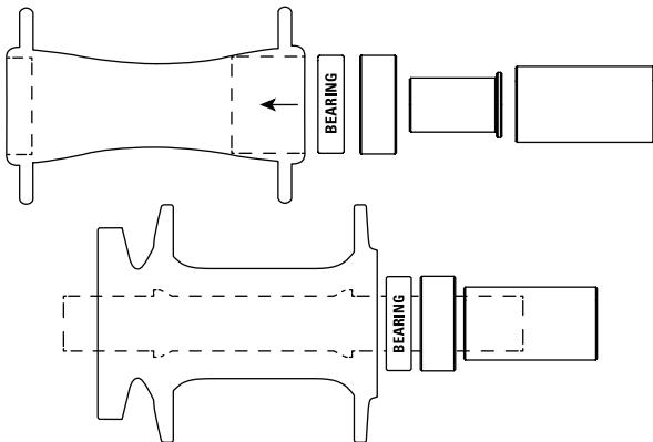
**EN 3. Select Spacer (if needed)** 4 spacers are included, each engraved with its ID and part number. The mechanic's judgement is required to determine if a spacer is needed. A spacer is typically used in situations when:
