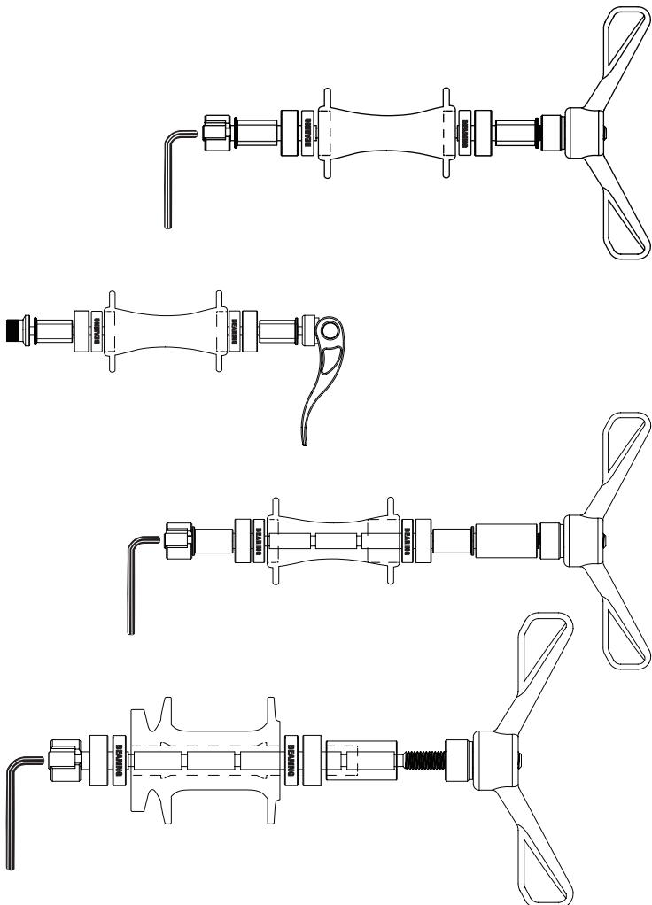
**EN 5. Assemble and Press** Assemble hub shell, bearings, bushings, pilots (if needed) and spacers (if needed). Examples of common assemblies are pictured in figures 5a - 5d. Slowly turn handle of press clockwise, making sure components stay aligned. Continue to turn handle until bearings are properly seated in hub. Do not overtighten.
