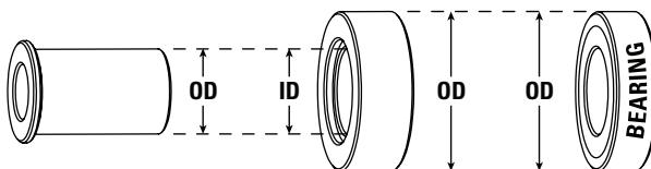
**EN 2. Select Bushing** The bushing presses on the outer surface of the bearing to prevent damage. 42 bushings (in 21 sizes) are included, each engraved with its ID, OD and part number. Select bushing with OD that matches OD of bearing and ID that matches OD of pilot and ID of bearing.
